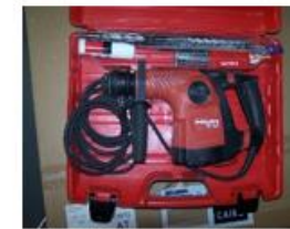
Hammer drill machine with metric driller of 16mm and 10mm (only during installation)
