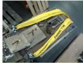
Tools to lift the equipment: Hoisting sling in different length 1 meter/3000kg, 3 meter/3000kg, 5 meter/5000kg
