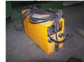
Electrical welding equipment
