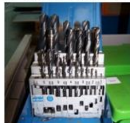
Drill bit metric 3-12mm (0,5mm steps)
